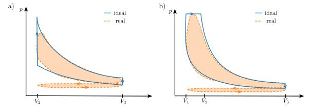
Figure 1: Schematic pV-diagram of the real and ideal Otto (a) and Diesel (b) cycle (color online).
